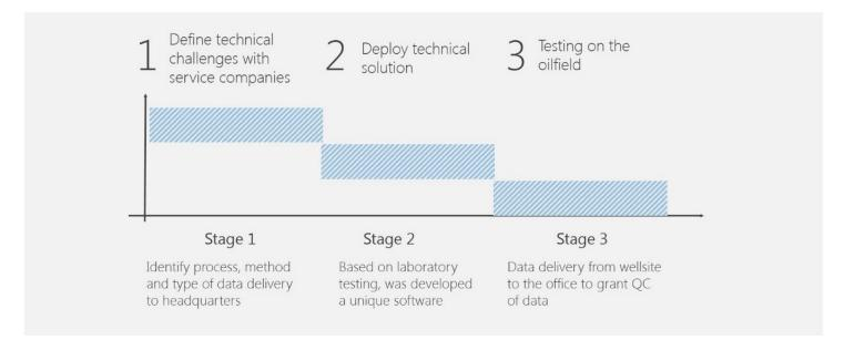
2 Software was developed that worked as a "coupler" to convert real-time ASCII data into the WITSML format. This software works in real-time, from our remote server integrator, allowing us to receive ASCII data in 2 different connection schemes, serial or Ethernet.
